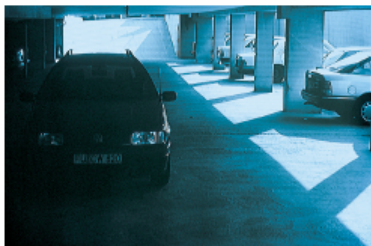
Fig. 3 Scene without backlight compensation and classification window
